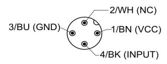
Colour coding only valid for coupling 4-poles mat. no. 1215497 and coupling 4-poles mat. no. 1262873
